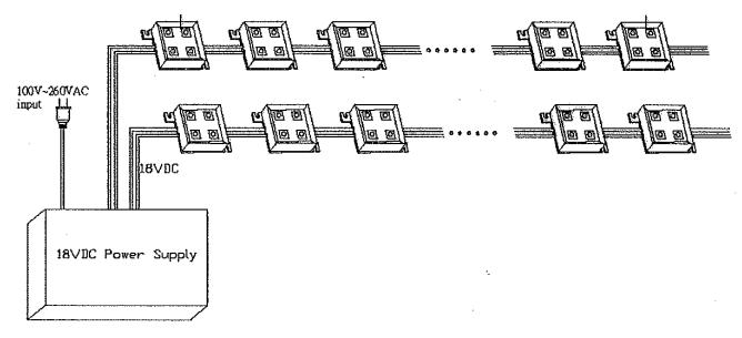
A twenty (20) LED Module string can be linked & driven with  $18V_{DC}$  as received out of the box. However, a maxium of 30 Red / Amber modules can be linked together in one serial string (Blue/Green/White up to 50 modules max in one serial string) with  $18V_{DC}$ . As many parallel strings that the power unit can handle is acceptable as long as the number of max modules stated above are linked in each serial string.
